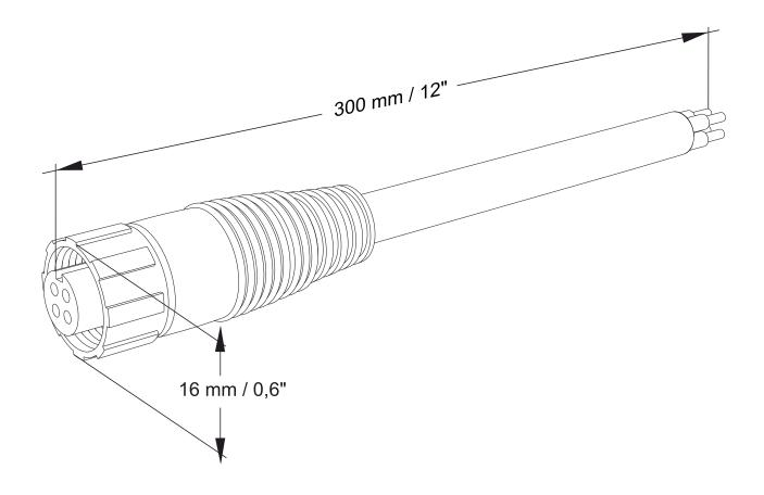
Ordering Code : P20027 4 Pin Female IP67 Cable & Connector 30cm
